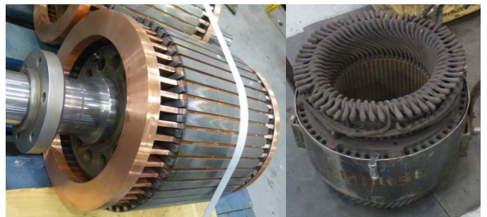
Fig. 1. 350 HP Railway traction motor (rotor & stator).
